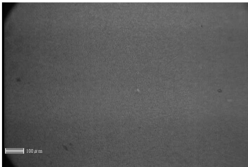
FIGURE 4 Photograph of the PBS solvent-cast film. Scale marker is 100 \mu\text{m} .
